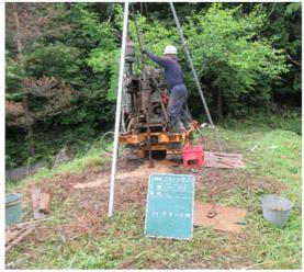
Embankment body investigation (boring investigation (standard penetration test))
